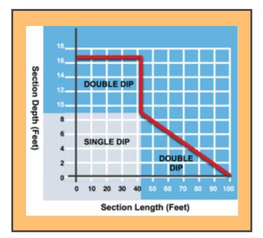
galvanized at our facility. The depth of section is indicated along the vertical axis and the corresponding maximum length is shown on the horizontal axis.
